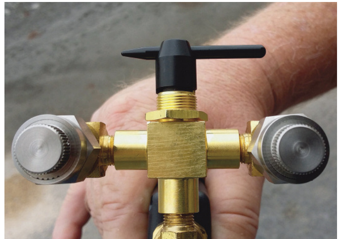
Photo 5 - THINVERT® applications require the use of specially-designed nozzles, such as this ULV Brush Gun with double nozzles. The nozzle on the left has 5 orifices and the right one has 31.
