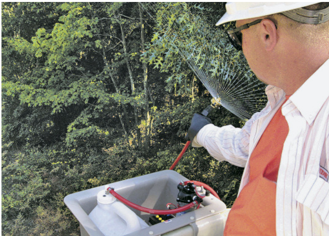
Photo 4 - Efficient and effective ULV side trimming can be accomplished with the THINVERT® application system mounted on the bucket of a 4-wheel drive lift truck or skidder.
